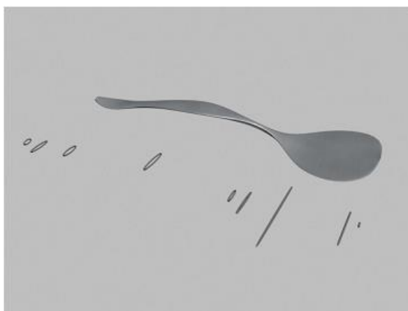
5.72-rasm. Create U Loft Surface buyrug‘idan foydalanib NURBS sirtini yaratish.
