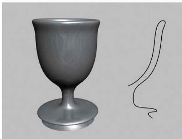
5.73-rasm. Create Lathe Surface buyrug‘idan foydalanib NURBS sirtini yaratish.
