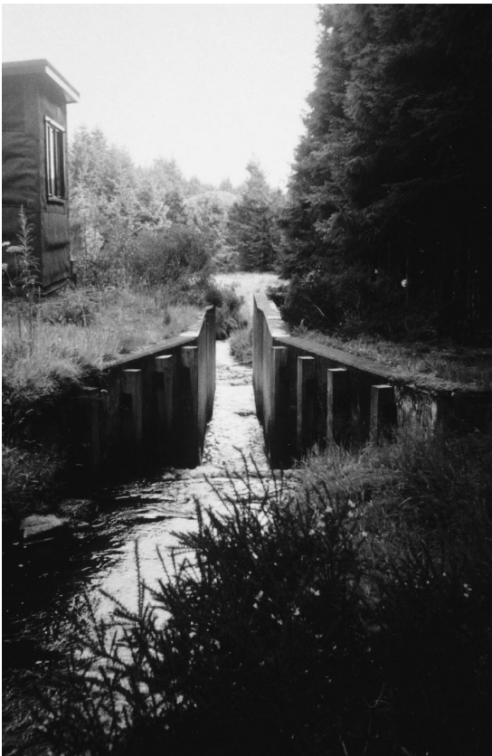
Figure 5.12 A trapezoidal flume. The stream passes through the flume and the water level at the base of the flume is recorded continuously.
